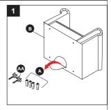
2. Remove the plastic caps on the threaded bolts of each leg. Attach wood legs with washers (A) to the bottom of the seat frame (B). Close the zipper.
