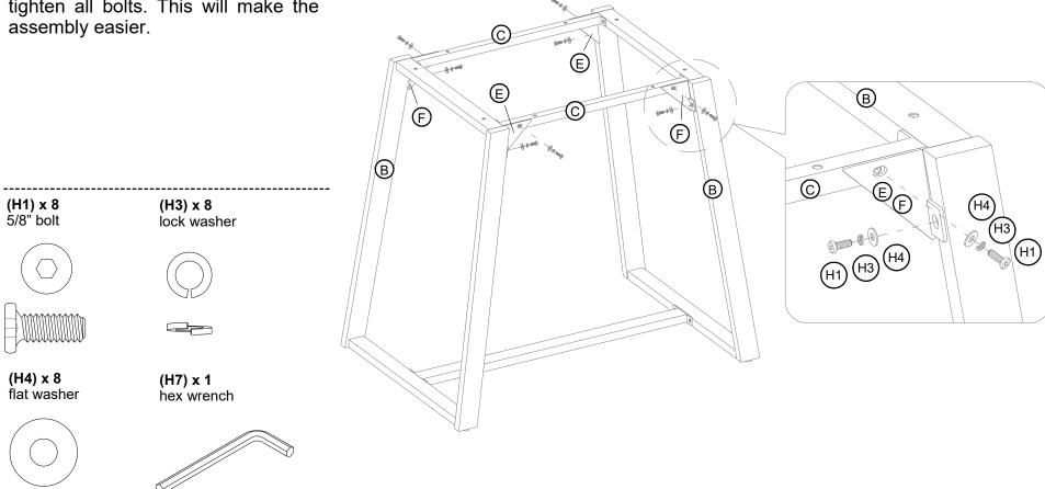
2.1. Align and attach the brackets (E and F) to the side frames (B) and both upper stretchers (C).
