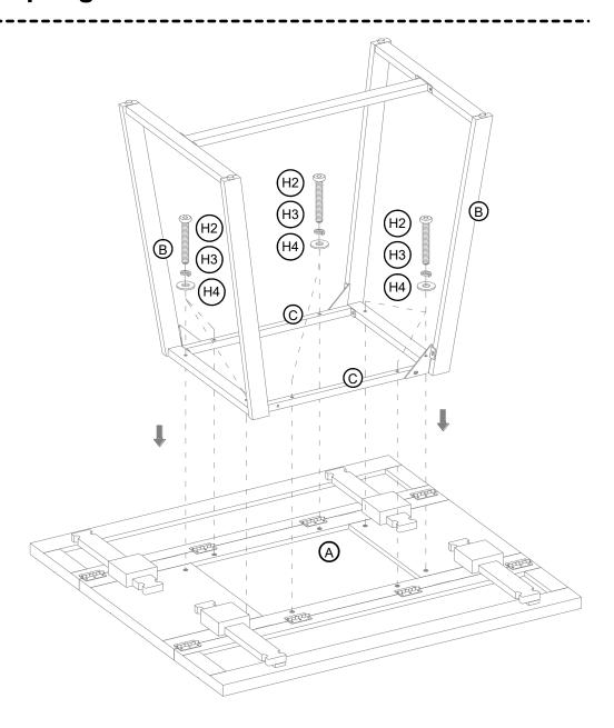
4.1. Flip over the assembled base and attach it to the table top (A).
