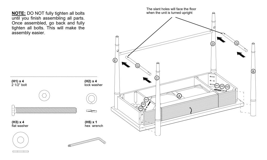
Attach the front legs (B and C) to the desk top (A) loosely and insert the side stretchers (G) between the legs properly.
