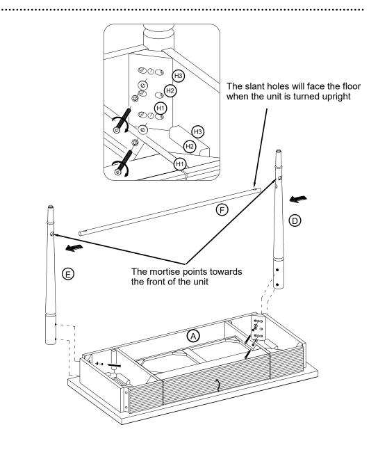
Fit the back stretcher (F) between the back legs (D and E) and attach them to the back apron of desk top (A).
