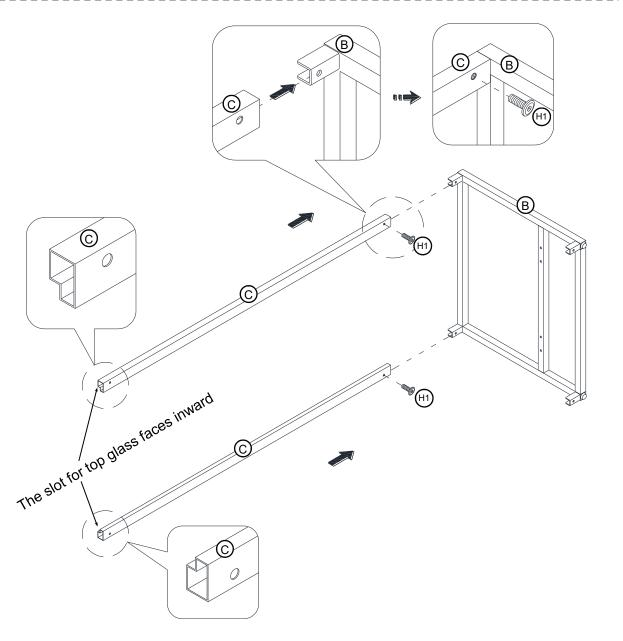
Align and attach the two top stretchers (C) to the top of one side frame (B).
