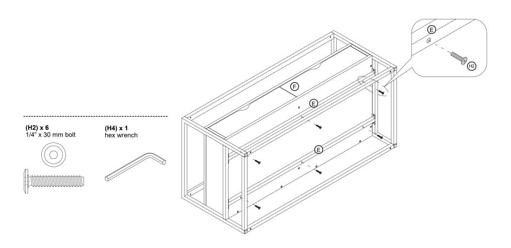
Firmly press the drawer box (F) against the drawer box supports (E). Make sure that the mounting holes overlap the threaded inserts underneath the drawer box (F) properly.
