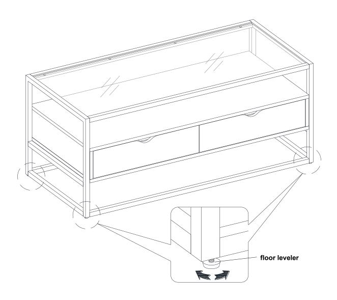
Position the unit at the desired location. If necessary, adjust the floor levelers to level the unit.
