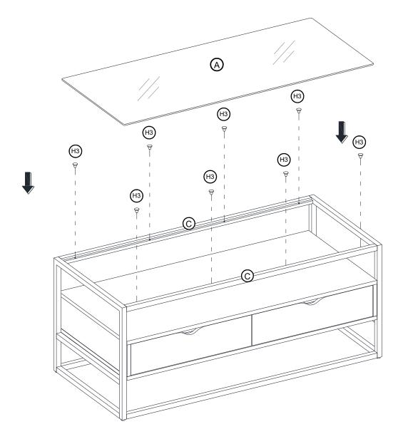
Stand the unit upright and firmly put the bumpers into the available holes on both top stretchers (C). Gently place the top glass (A) onto the bumpers on the slots of top stretchers (C).
