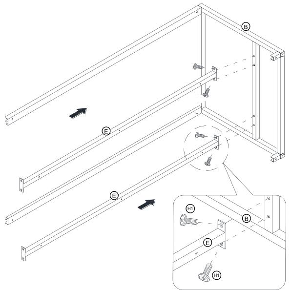
Fasten the two drawer box supports (E) to the middle rail of side frame (B).
