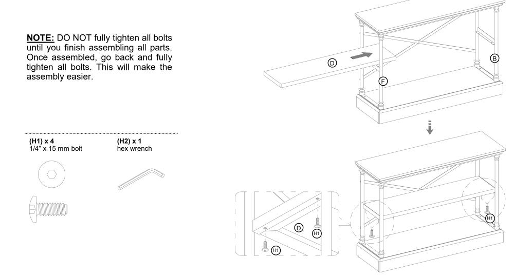
4.1. Attach the middle shelf (D) to the middle rails of the side frames (B and F) using four 15 mm bolts (H1).
