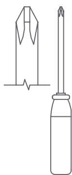
No. 2 Cross-head Screwdriver Tip Shown Actual Size
