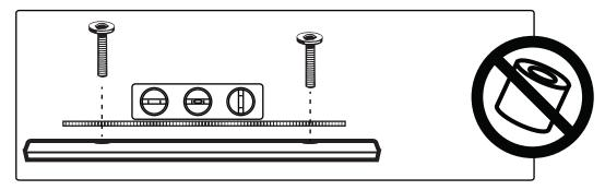
• **Obstructed back**: The brackets block any of the jacks on the back of your TV. You will need spacers when assembling the wall mount.
