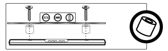
• Irregularly-shaped back: There is a gap between the bracket and some part of the back of your TV. You will need spacers when assembling the wall mount.
