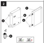
Lift seat frame (D) on the open end where hooks are located and let the downward facing hooks (b) slide into the upward facing hook slots (a) located on the inside of armrests (B).
