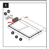
Remove the plastic caps on the threaded bolts of each leg. Attach wood legs with washers (A) to the bottom of the armrests (B & C).
