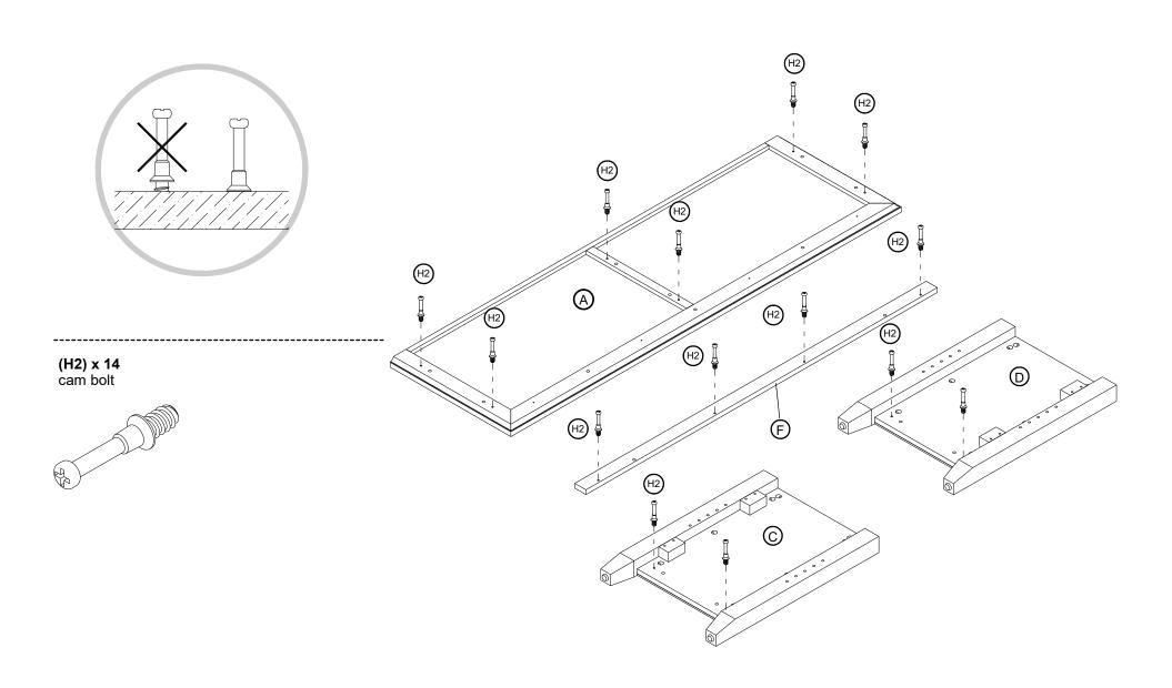
Screw-in the cam bolts on top panel (A), bottom front molding (F) and the legs (C and D).
