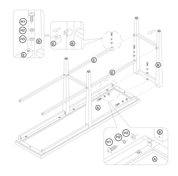
7.1. Align and attach one side frame (B) to the previous assembly with five 15 mm bolts (H1) and five washers (H2 and H3).
