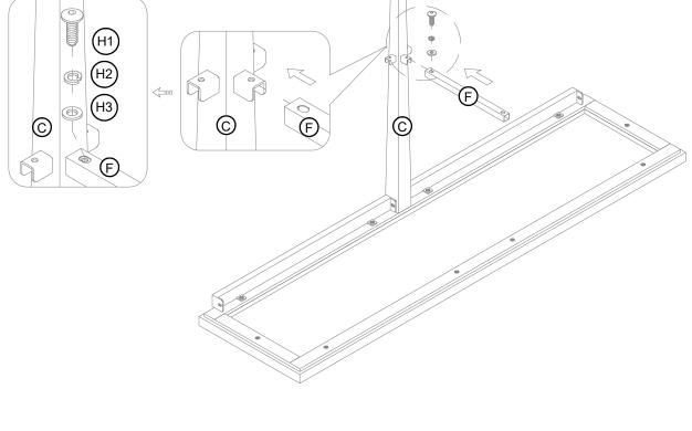
3.1. Orient and fit the middle stretcher (F) onto the U-shaped bracket on the assembled middle leg (C) and secure it into place with one 15 mm bolt (H1), one lock washer (H2) and one flat washer (H3).
