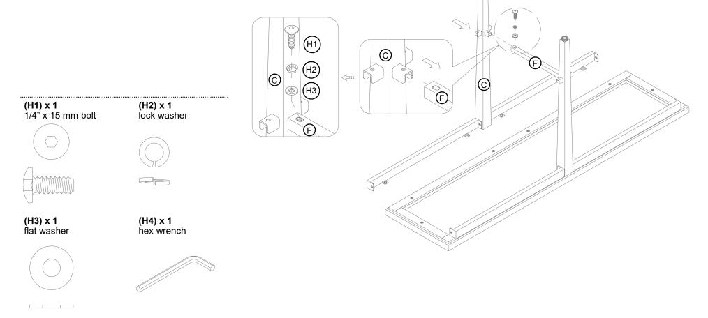
4.1. Repeat the same process to attach the other assembled middle leg (C) to the other end of the middle stretcher (F). Make sure that the metal tabs overlap the threaded inserts on top panel (A) properly.
