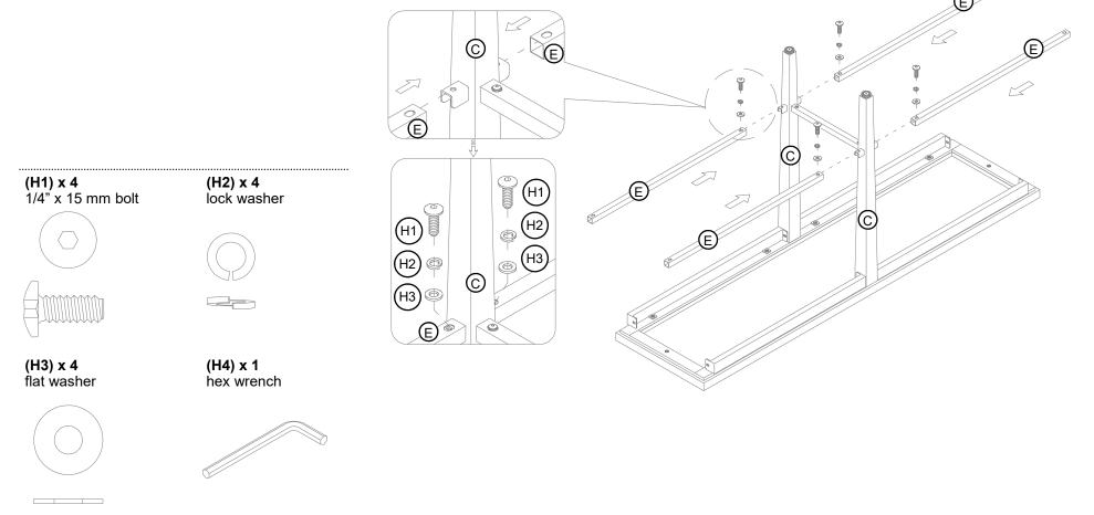
6.1. Orient and fit the bottom stretchers (E) onto the U-shaped bracket on the assembled middle legs (C) and secure into place with four 15 mm bolts (H1) and four washers (H2 and H3).
