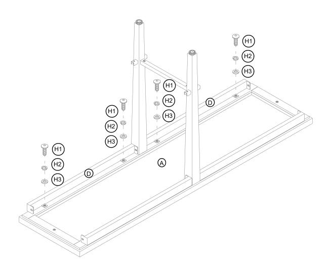
5.1. Insert four 15 mm bolts (H1) with washers (H2 and H3) through the metal tabs on the assembled top stretchers (D) and screw into the top panel (A).
