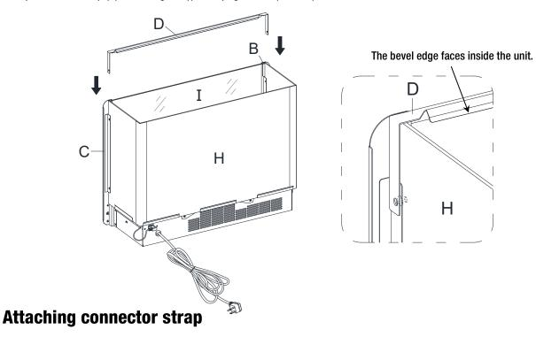
□ Fasten connector strap (D) to both upright arms (B and C) using two screws (AA) as show below. Holes must be in line for screw to pass through.
