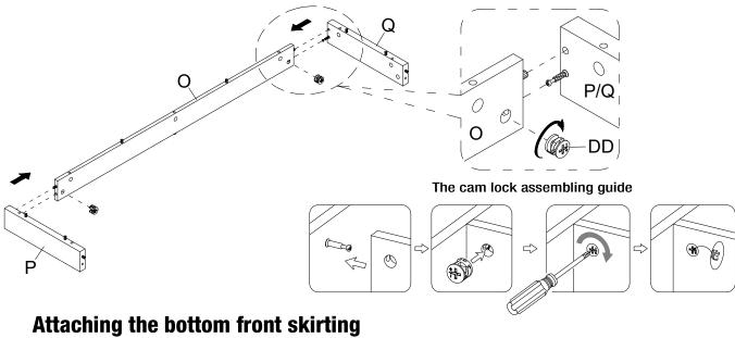
Attach the front skirting (N) to the side skirtings (P and Q) by engaging two cam locks (DD).
