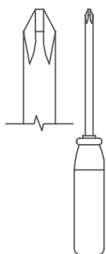
No. 2 Cross-head Screwdriver Tip Shown Actual Size
