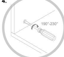
Rotate cam(s) clockwise 190°-230° to lock panels together
