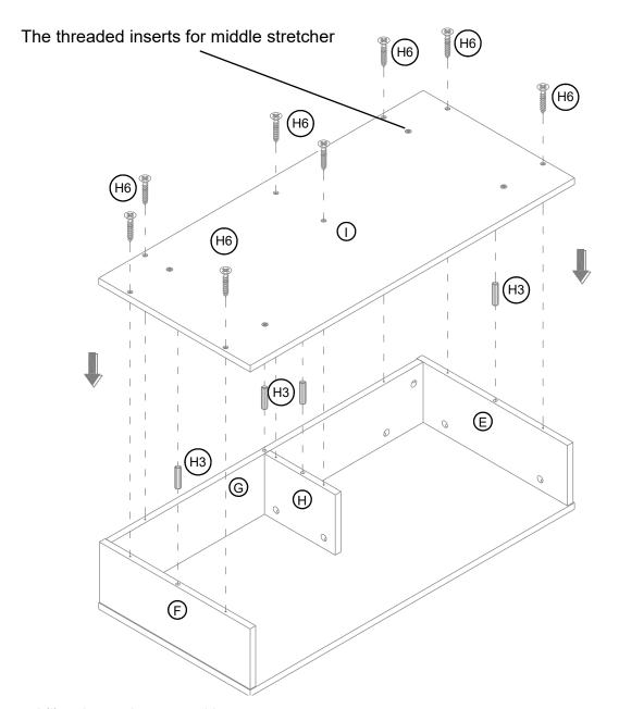
5.1. Using the pilot holes as a guide, attach the compartment bottom panel (I) to the previous assembly.
