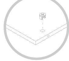
Push cam into panel - arrow feature on cam top points to panel edge
