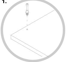
Screw cam bolt into panel
