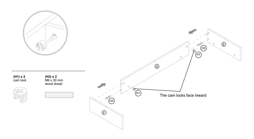
2.1. Attach the back panel (G) between the side panels (E and F).
