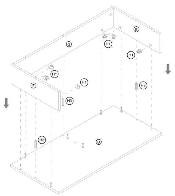
3.1. Attach the previous assembly to the compartment top panel (D).
