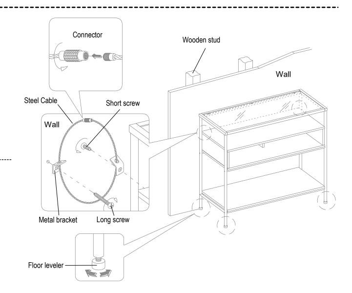
Tools required: Phillips screwdriver, stud finder, tape measure, pencil, power drill and 1/8" drill bit.
