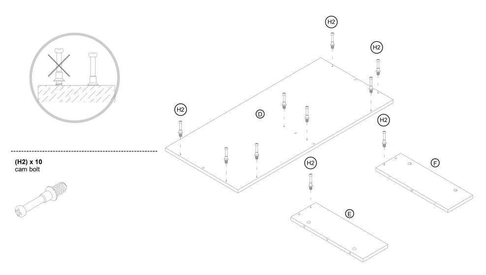
1.1. Screw-in the cam bolts on the compartment top panel (D) and the side panels (E and F).
